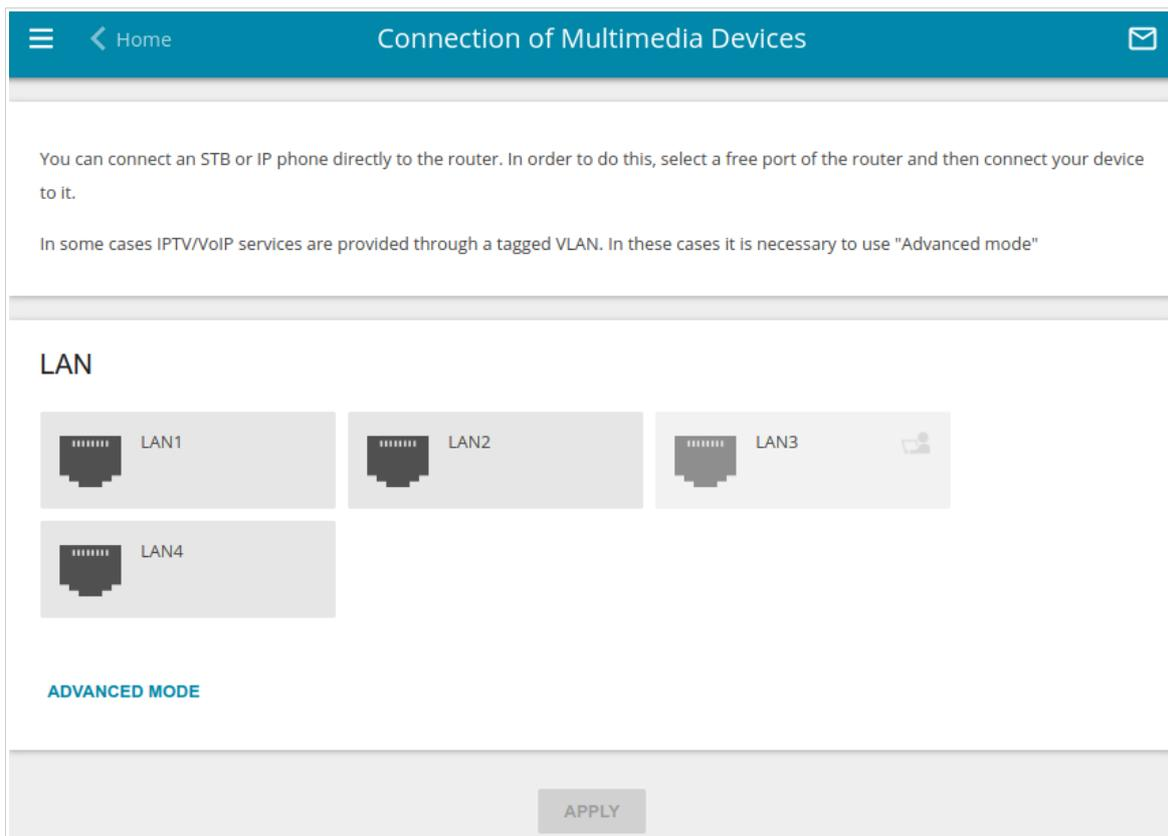
Figure 53. The Multimedia Devices Connection Wizard. The simplified mode.
