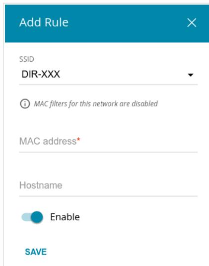
Figure 108. The window for adding a rule for the MAC filter.
