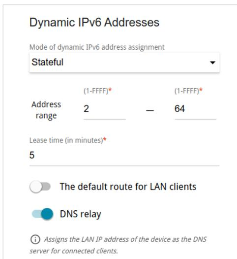
Figure 90. Configuring the local interface. The IPv6 tab. The **Dynamic IPv6 Addresses** section.
