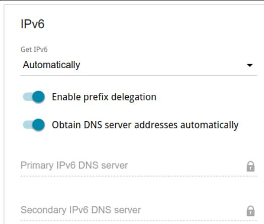
Figure 81. The page for creating a new PPPoE Pv6 connection. The IPv6 section.
