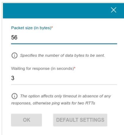
Figure 147. The **System / Ping** page. The additional settings window.
