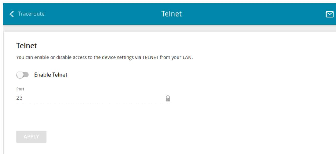
Figure 150. The **System / Telnet** page.
