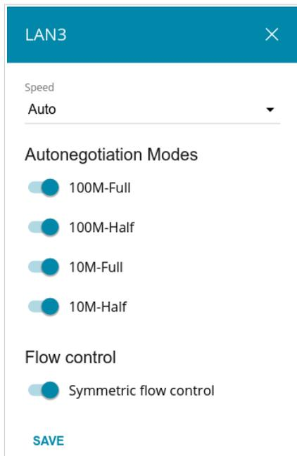
Figure 119. The window for changing the settings of the router's port.
