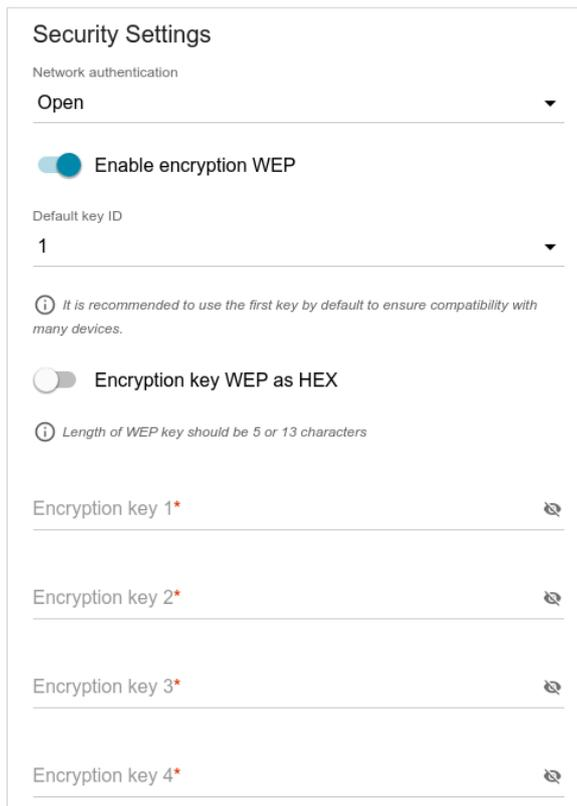
Figure 98. The **Open** value is selected from the **Network authentication** drop-down list.
