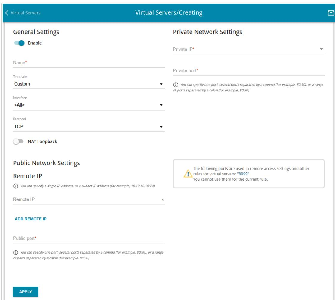
Figure 132. The page for adding a virtual server.
