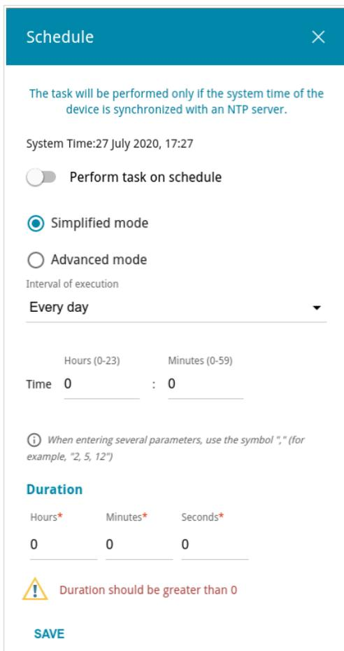
Figure 143. The window for adding a schedule for a task.
