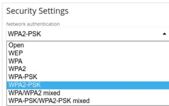
Figure 97. Network authentication types supported by the router.
