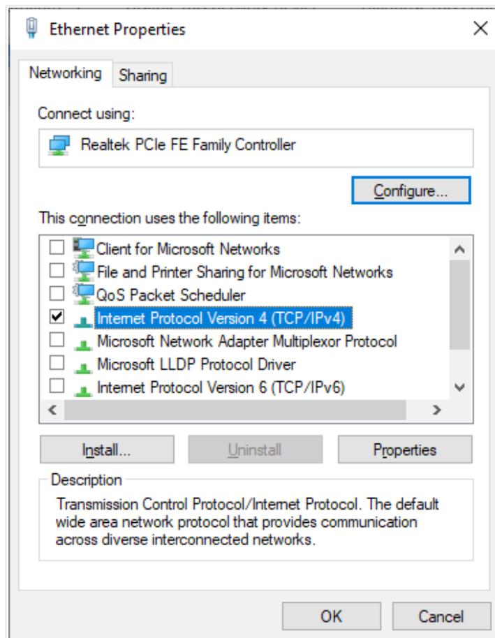
Figure 12. The local area connection properties window.
