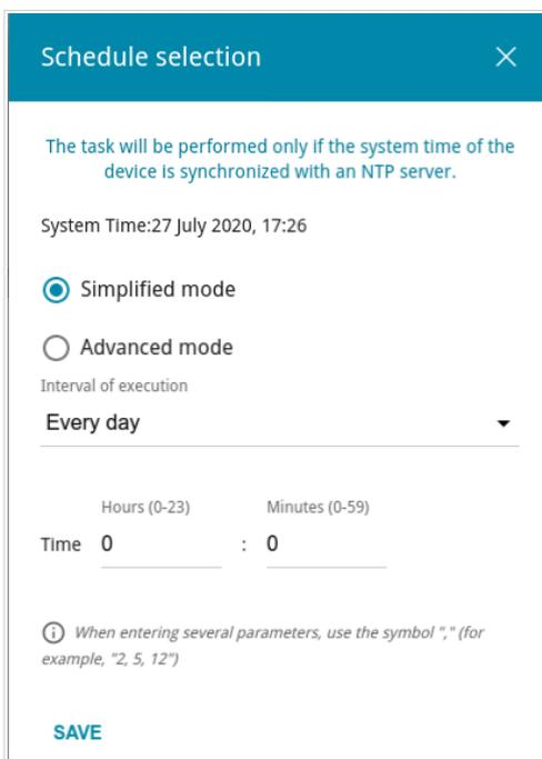
Figure 142. The window for configuring automatic reboot on a schedule.
