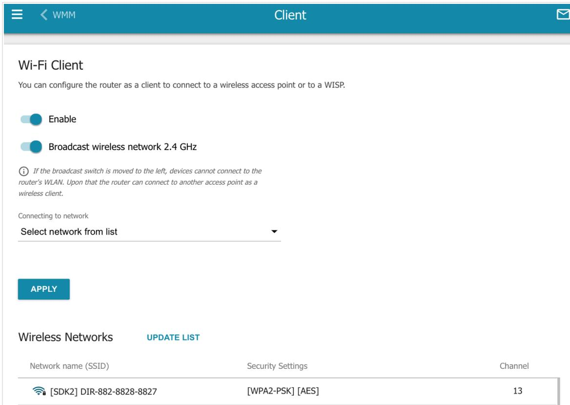
Figure 105. The page for configuring the client mode.
